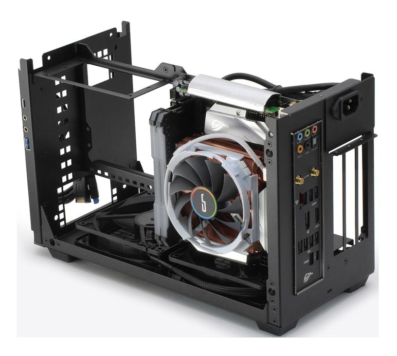
It is recommended to install your CPU, RAM, and CPU cooler onto your motherboard before placing the motherboard into the case.
