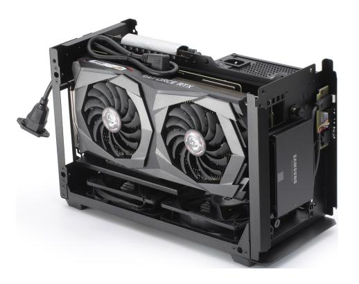
PCIe cards are secured with up to 3x M3 PAN HEAD screws.
