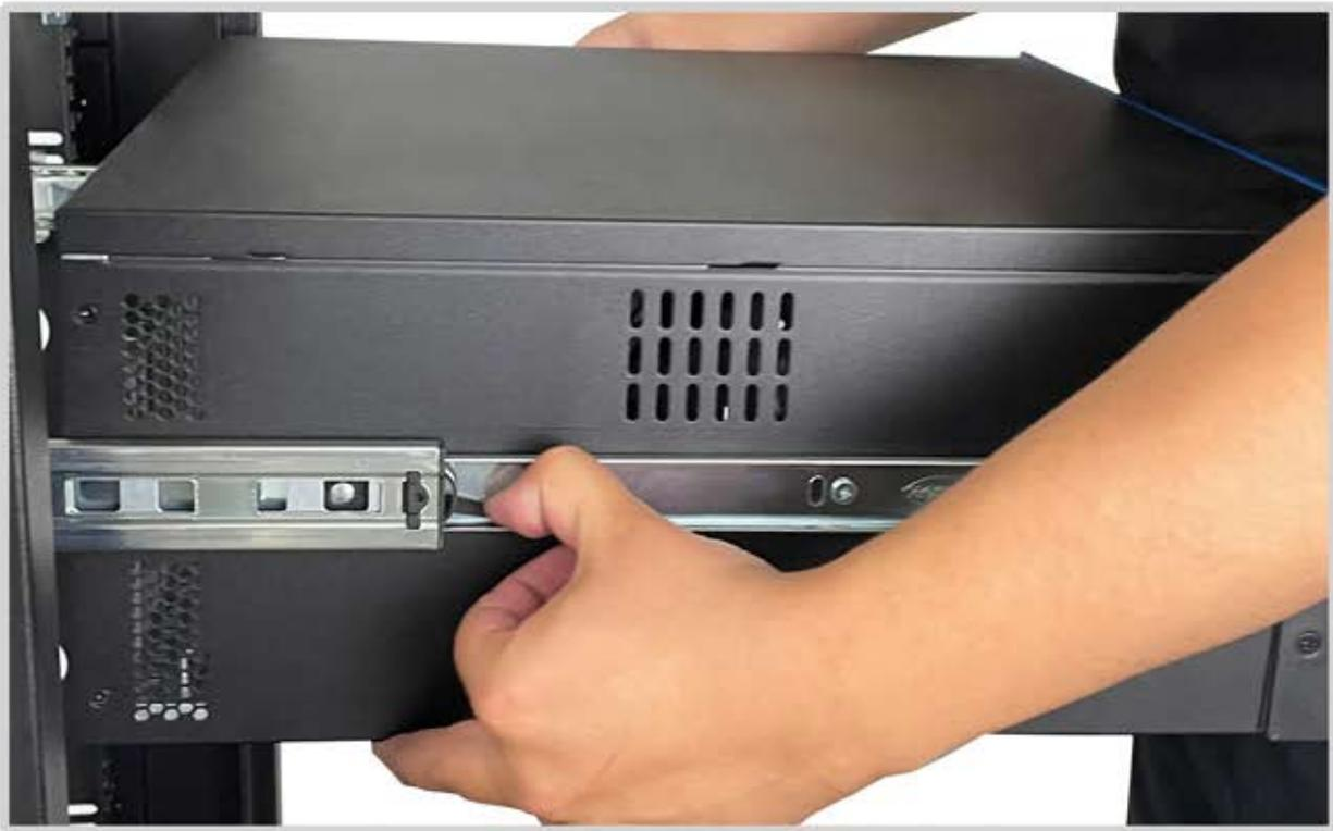
Once the inner slides are successfully centered and slide into the middle members, you will need to press down the security latches to finish sliding the chassis into your rack cabinet.
