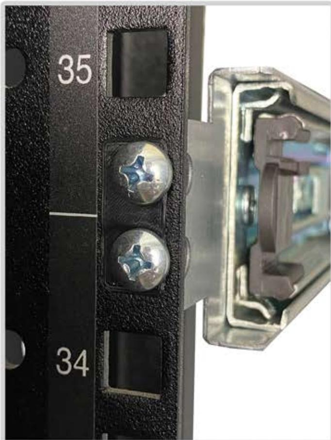
Once the screws are both in place, tighten down both screws.
