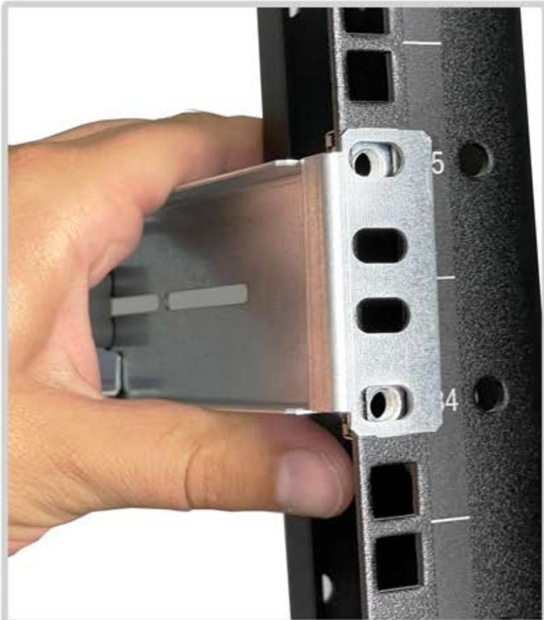
The side of the screw vs the side of the nut does not matter. If it is easier to put the screw on the inside, put the screw on the inside.
