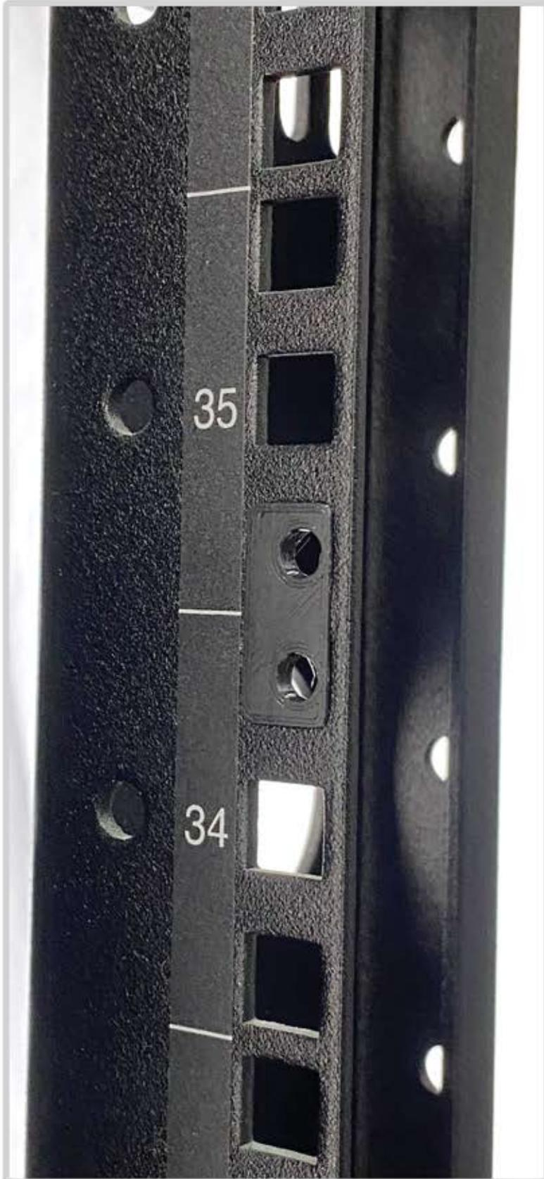
Install the Front Offset Clips as pictured, with screw pass-through holes offset to inside of rack cabinet.
