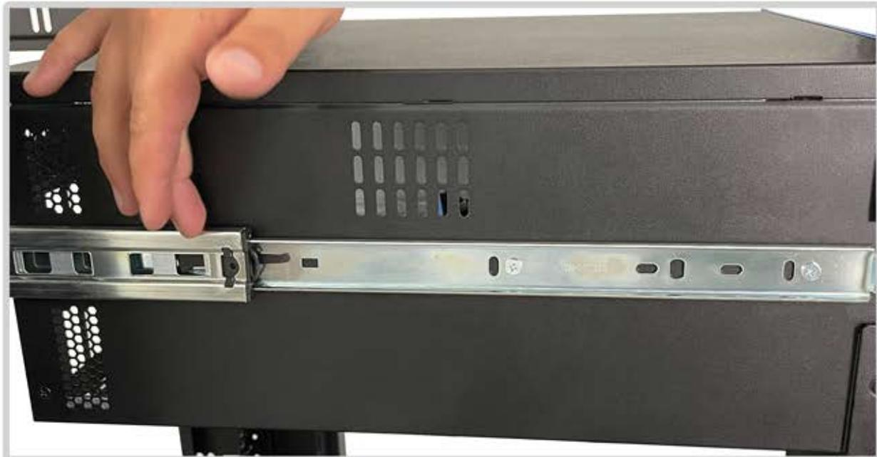
**NOTE:** It may take more than one attempt to get the chassis to line up with both slides. The chassis should slide almost effortlessly once properly installed in the slides. If there is friction, remove and try again.
