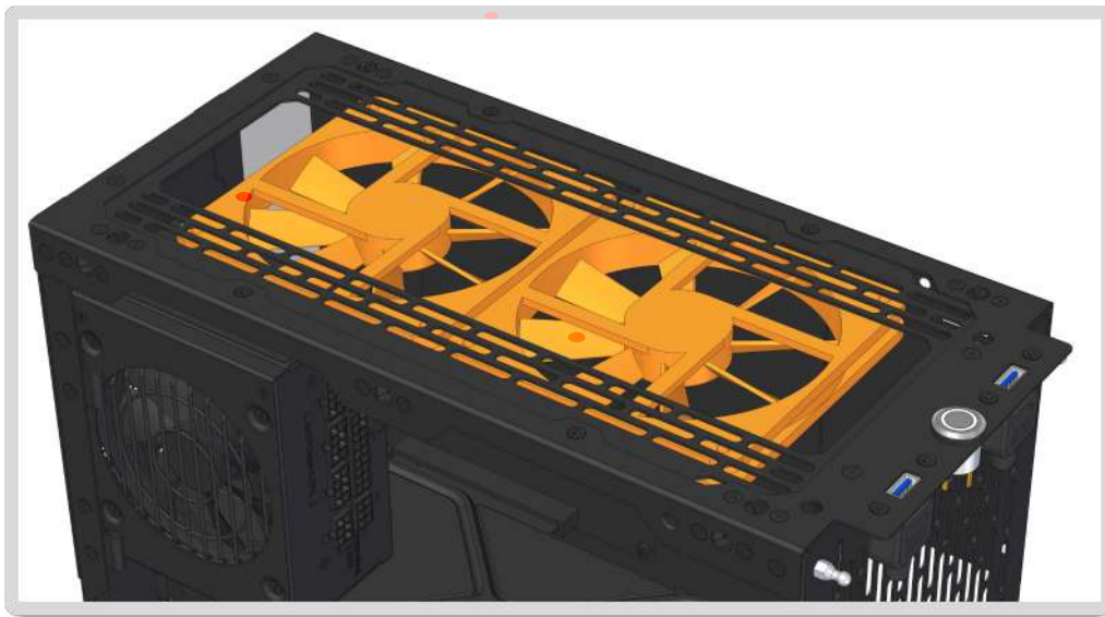
120mm x 15mm Fans mounted to Sub Top Bracket
