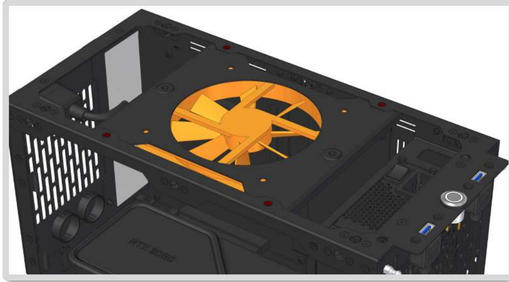
120mm x 15mm Fan mounted to Handle Bracket
